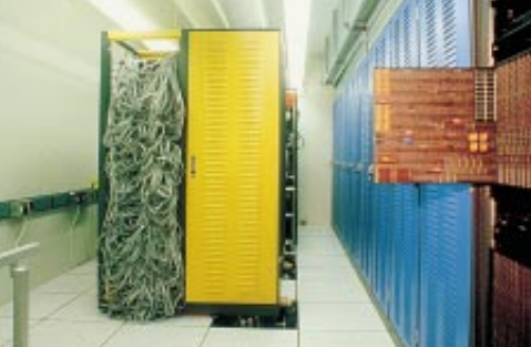
GF11 SUPERCOMPUTER consists of 566 parallel processors. The "permuter" collects and feeds data to the processors, and the controller orchestrates all the activity. In the photograph, the processors are the bronze panels that slide into racks; the cables belong to the permuter-controller system.
